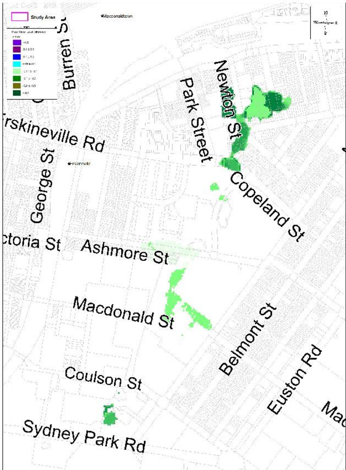
Figure D3 20 Year ARI Peak Water Level Difference for FM5 Less Existing
