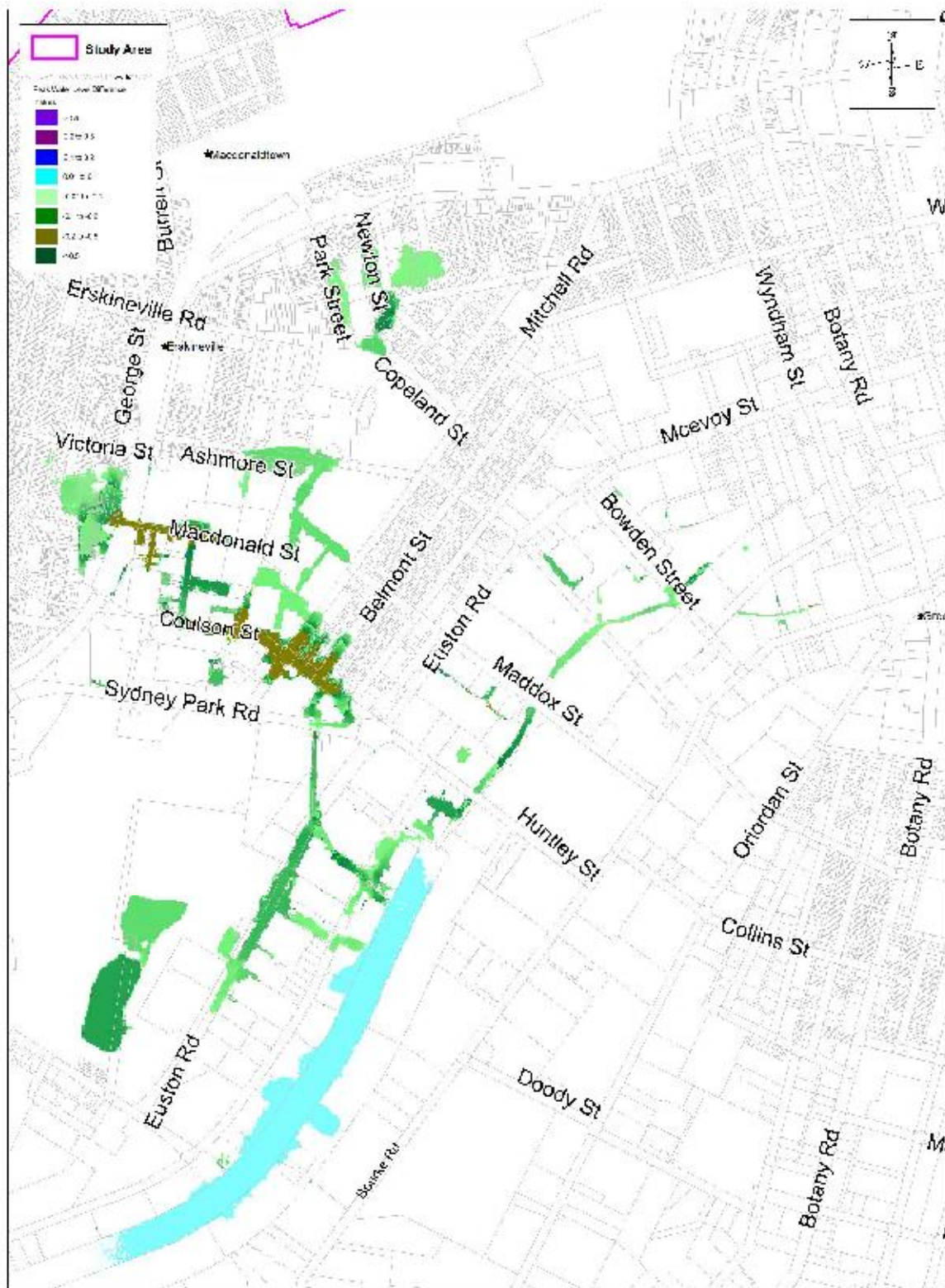
Figure D6 20 Year ARI Peak Water Level Difference for FM6 Less Existing
