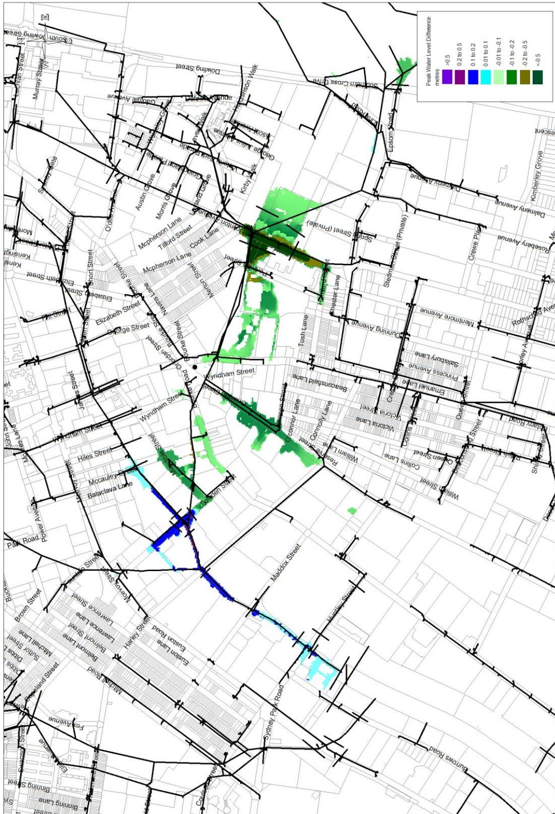
Figure F4 100 Year ARI Peak Water Level Difference for FM2 Less Existing
