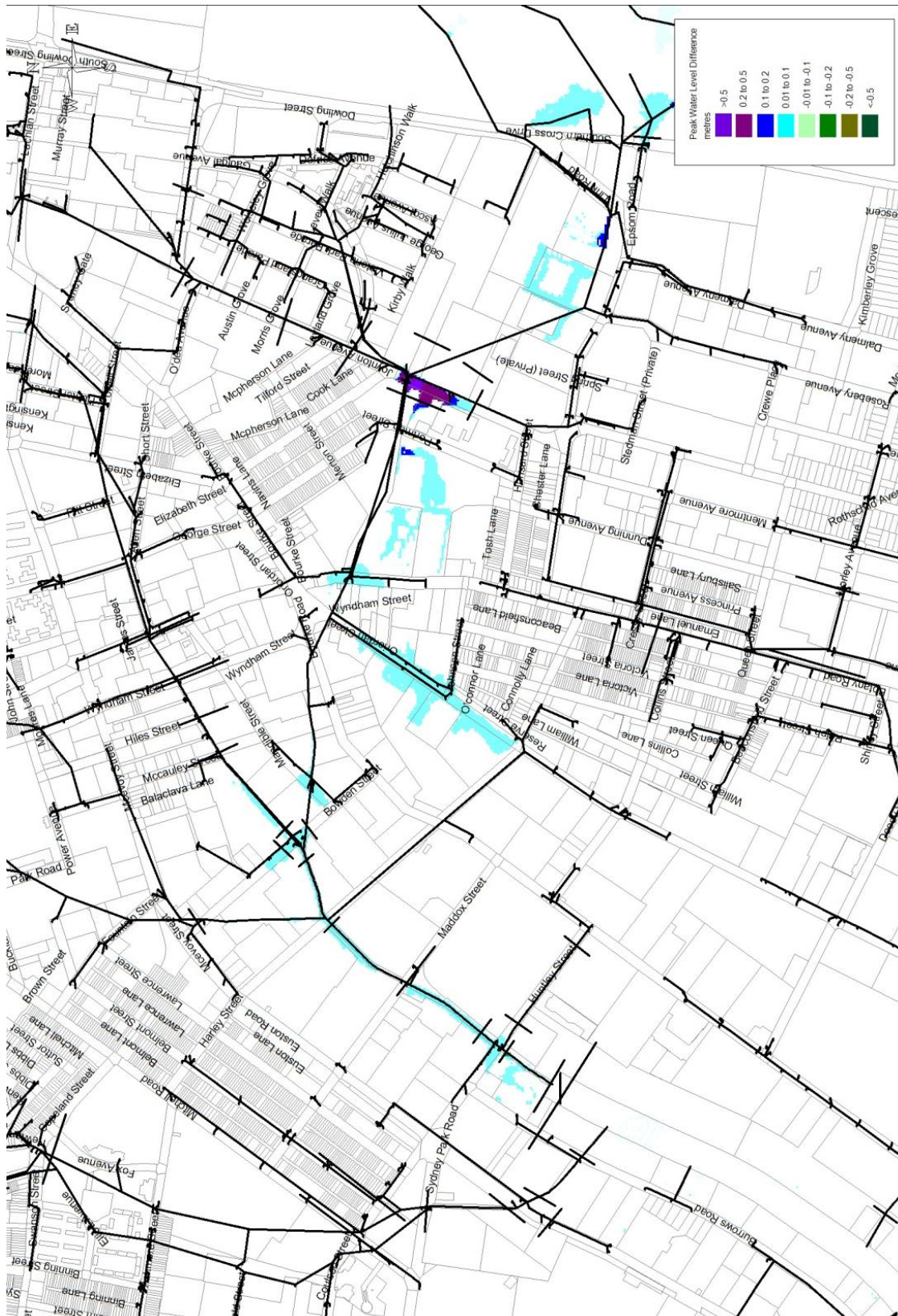
Figure F6 100 Year ARI Peak Water Level Difference for FM4 Less FM3
