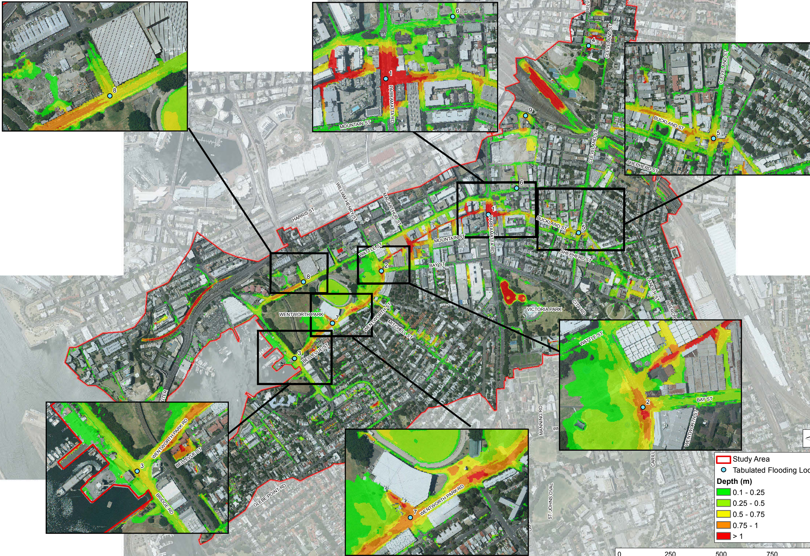
FIGURE 28 ACCESS ROAD FLOODING 1% AEP DESIGN FLOOD EVENT
