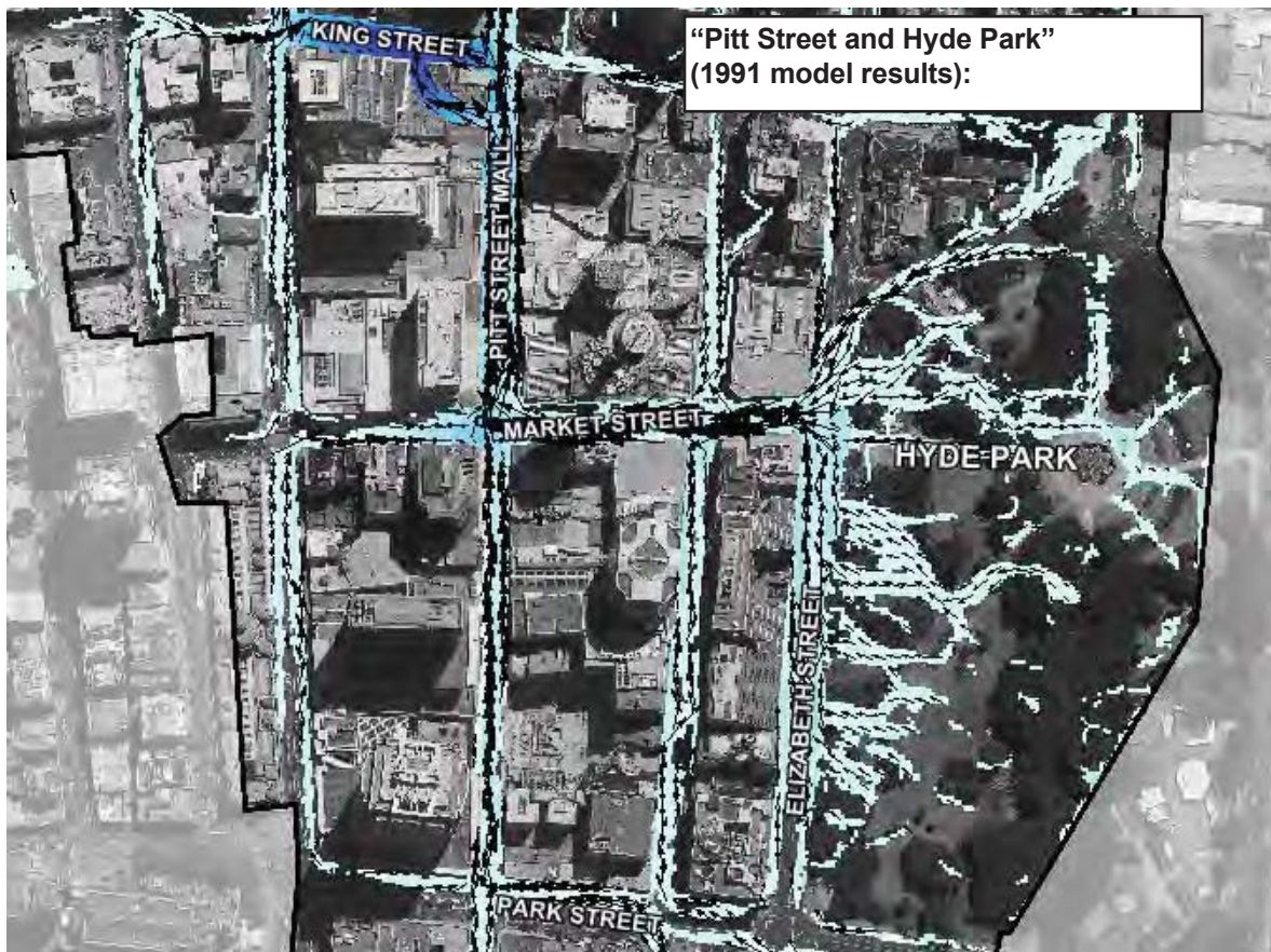
Figure 5-12 Historic flooding reports on Pitt Street and from Hyde Park
